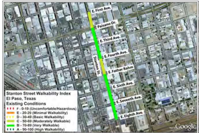
Walkability Index Results for Stanton Street in Downtown. The solid chartreuse line signifies a grade of C, or Moderately Walkable. The solid green line signifies a grade of B, or Very Walkable.
