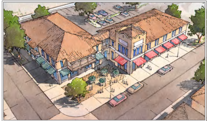
Version 1: This placita , or small plaza, configuration is ideal for corner sites. The two buildings are offset subtly to create a usable open space. An arched walkway provides pedestrian access from the rear parking lot, while connecting the buildings on their upper floors.
