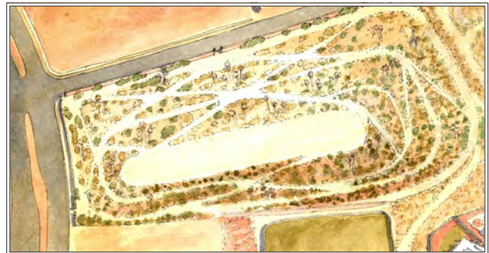
An alternative to the conventional drainage basin creates habitat through the use of native plant species while still performing stormwater duties.
