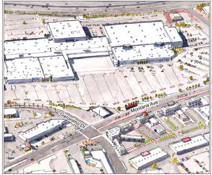
Step 1: Crosswalks, bus shelters, and a designated transit lane begin to make Montana Avenue more hospitable to the RTS and its riders. A corner gas station can be reconfigured as a “gas backwards,” as illustrated previously on page 2.34.
