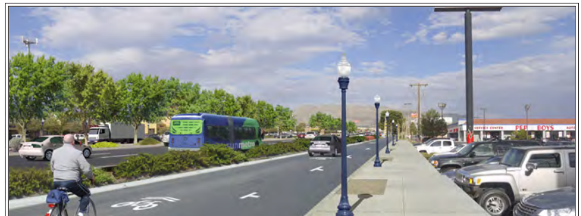
STEP 1: Mesa Street is converted to a multiway boulevard. Street trees, a central median, slip lanes, bike lanes, and parallel parking are added, and bus stops are incorporated along the outer medians. Paved sidewalks and dignified lighting replace gravel landscaping along the edge of parking lots.
