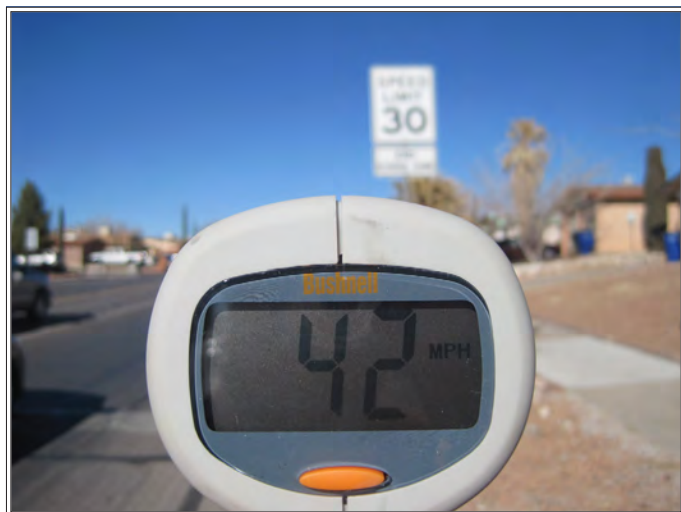
One part of the Handlebar Survey involves recording vehicular speeds to determine the safety of streets for bicycling.
