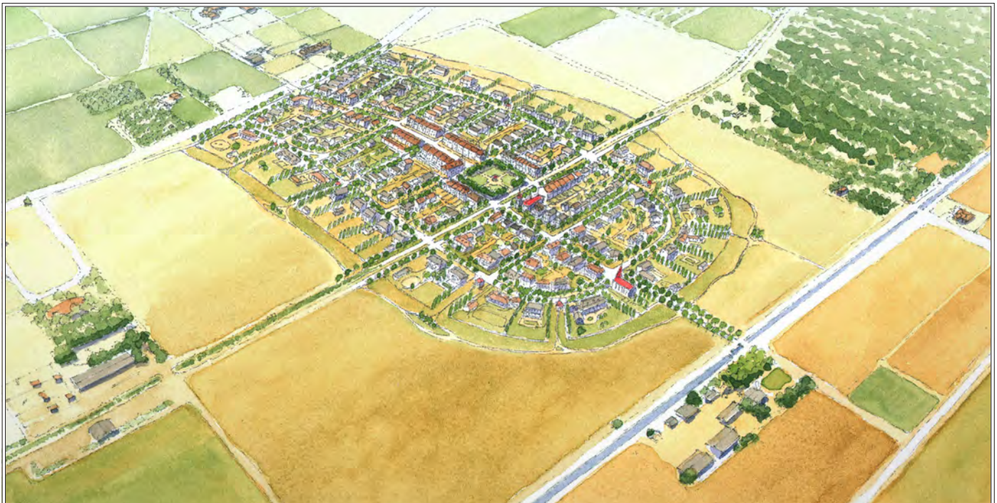
Example of Clustered Development in the Upper Valley: By allowing the same 225 permitted units to be clustered on a portion of the square quarter-mile, the remainder of the site could be preserved in perpetuity as usable agricultural land.
